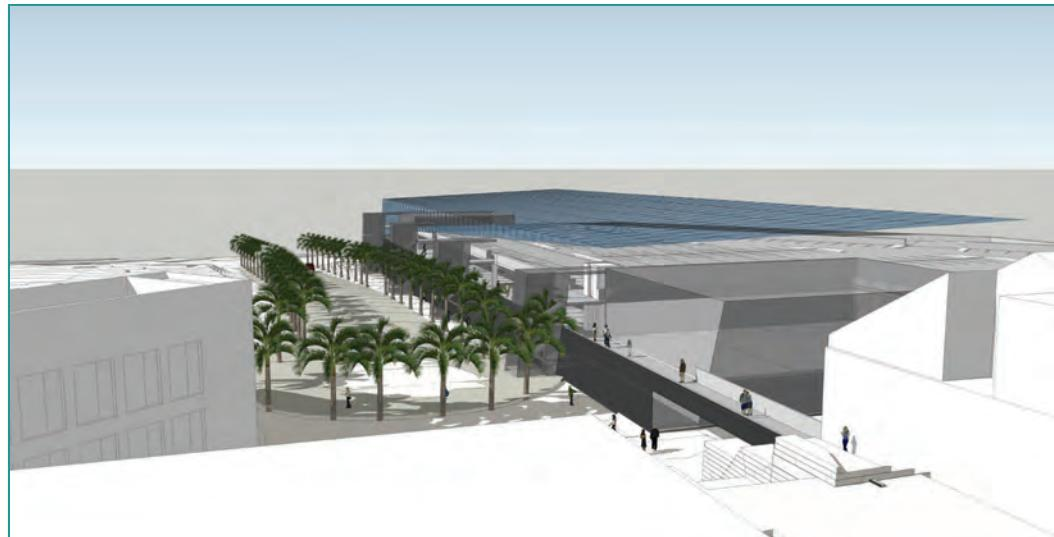
*This drawing shows the parking structure from an aerial perspective. The blue shaded area is an immense solar panel that will be somewhat see through. This panel will harness the sun’s rays to create enough energy to supply the entire structure, as well as surface lighting for all campus parking lots. As an added benefit, the solar panel will provide shade for a portion of the top level of the structure.*
