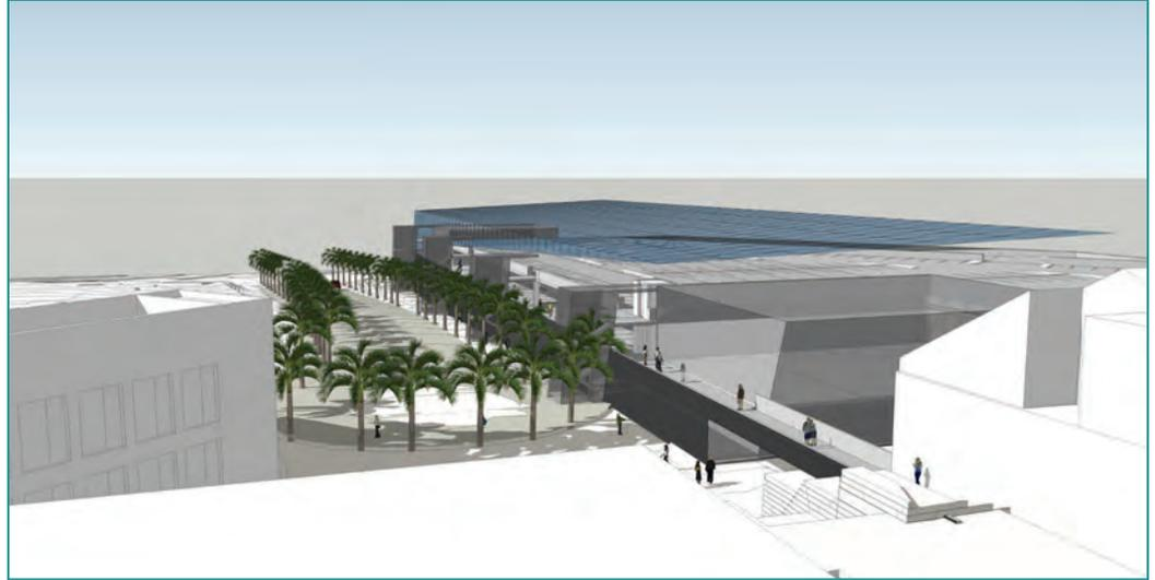
*This drawing shows the parking structure from an aerial perspective. The blue shaded area is an immense solar panel that will be somewhat see through. This panel will harness the sun’s rays to create enough energy to supply the entire structure, as well as surface lighting for all campus parking lots. As an added benefit, the solar panel will provide shade for a portion of the top level of the structure.*
